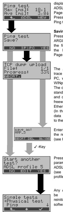
display the ADSL mode, ADSL line parameters... (see Page 29). . Press <**NEW**> to start a new Ping test.
