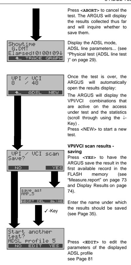
Any ADSL test desired can be started without reinitializing the ADSL test software.
