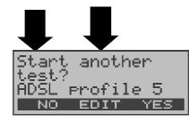
Press **<EDIT>** to edit the parameters of the displayed ADSL profile (see "Configuring ADSL profiles" on page 81 )
