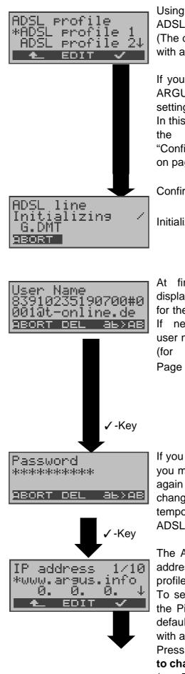
Using the  $<\downarrow>$ , select an ADSL profile. (The default profile is marked with an "\*".)
