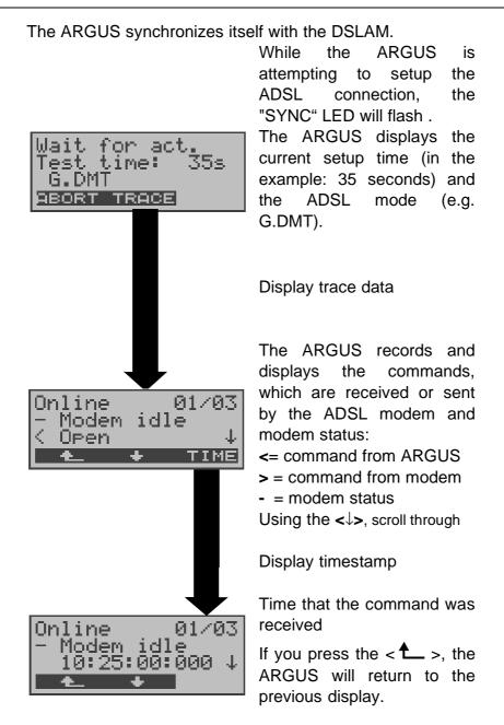
If the connection is not successfully setup within a specific time (a maximum of 2 periods of 4 minutes = "Time out") or if an error occurs during the setup, the ARGUS will display a corresponding error message (see "Error message: ADSL connection" on page 111):
