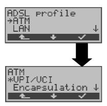
In addition to the physical parameters (Physic. line), Bridge mode also requires that the two ATM parameters - VPI/VCI (Page 90) and - Encapsulation (Page 90) be set.
